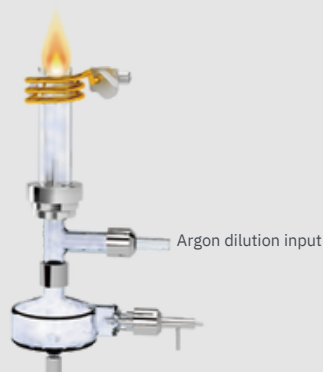
Schematic diagram for argon dilution input
